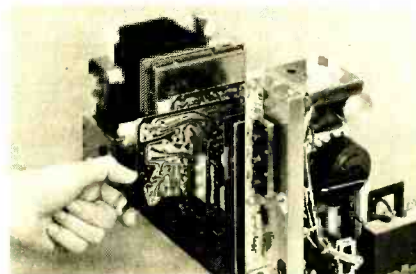
THE SEVEN MODULES of the Admiral ERA II can be changed in seconds.
